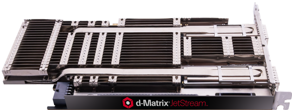
Figure 1. d-Matrix JetStream: purpose-built ultra-low latency Transparent NIC
